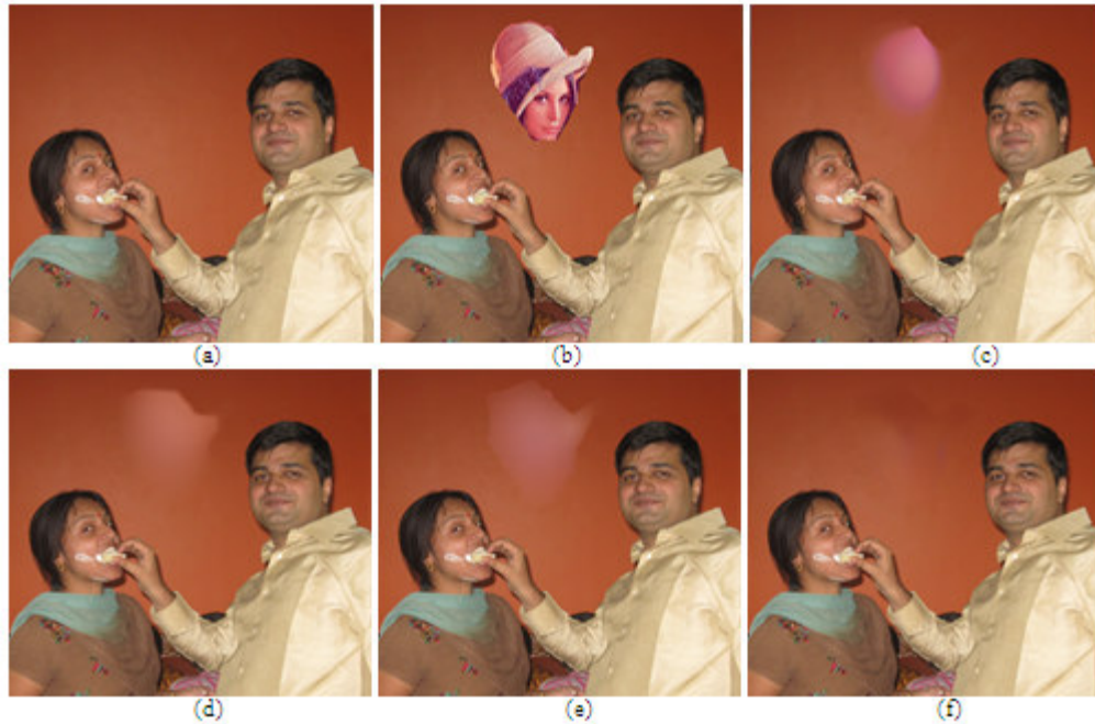
Figure 5 Inpainting Lena's face placed on pair image. (a): Clean undamaged pair image. (b): A sub image (Lena) is placed on clean image. (c): Bertalmio's technique (PSNR=25.7076 dB). (d): FoE technique (PSNR=31.9746 dB). (e): Gaussian pyramid technique (PSNR= 31.63 dB). (f): Proposed hybrid approach with PSNR=44.5434 dB.
